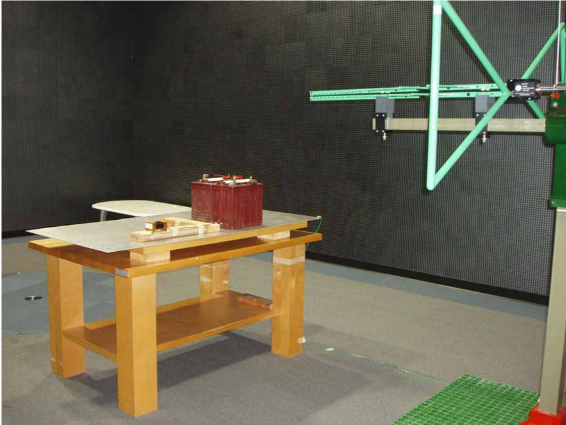
Photo 1 – Radiated Emissions Test Set-up
